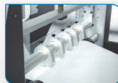
Heavy Duty Slitting Station Slit media down to size with inline slitting
